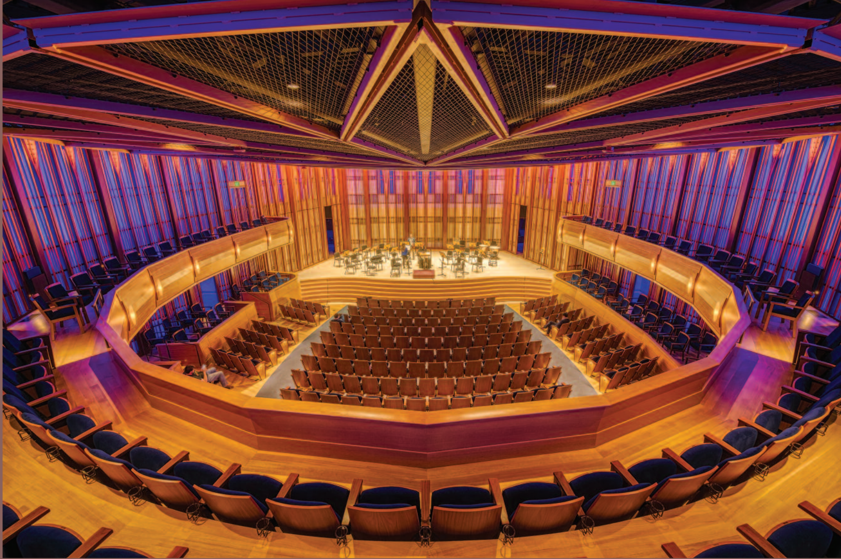
Above and opposite: "We combined the shoebox and opera forms," Joslin says of the Baker-Baum. Surrounding the attractively curved horseshoe auditorium is a concrete shoebox. Separating them is a wood lattice, which defines the room visually and has acoustical implications. "The sound goes through the slatted walls and meets the concrete of the shoebox."
